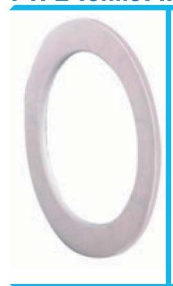
Pure PTFE gasket reinforced with a perforated stainless steel 304 insert, easy installation, cold flow is limited by the insert. Universally chemically resistant, acids and alkalis. For temperatures -100 up to +250 °C.
